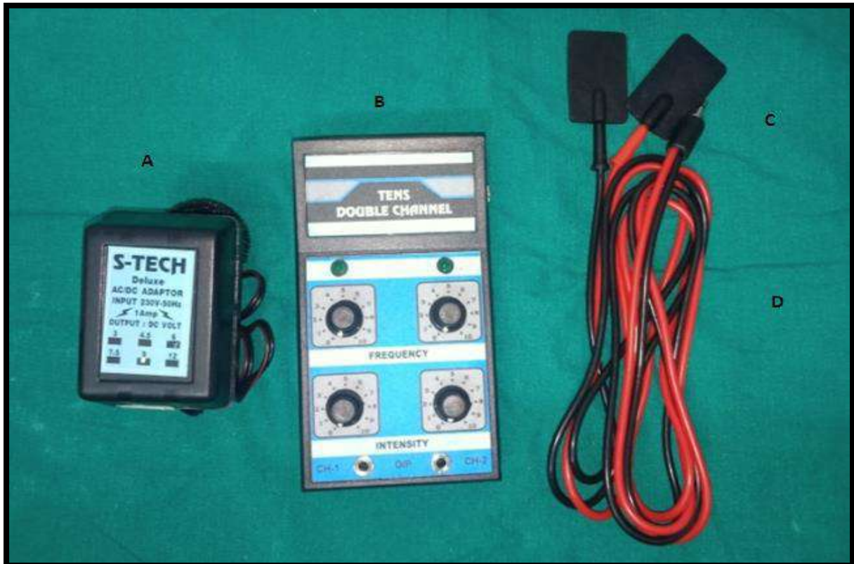
Figure no 1: TENS unit A) Adaptor B) TENS unit C) Electrodes D) Lead wire
