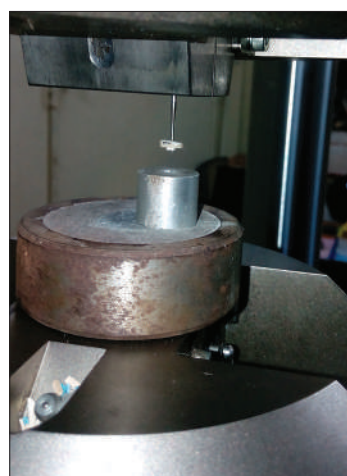
Figure 3: Universal Testing Machine containing cylindrical stainless steel plunger of 1-mm diameter and operating at a speed of 1 mm/min -1 used to apply force on materials, inside root slices.
