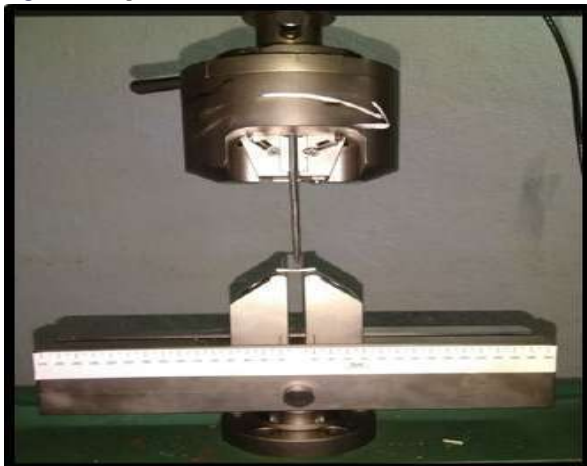
Figure 3: Testing Of Samples Under Universal Testing Machine
