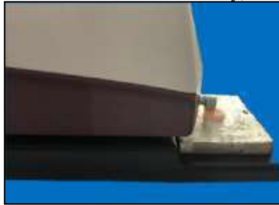
Fig no 3 Measuring surface roughness with surface roughness tester (Mitutoyo)
