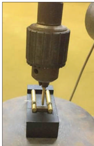
Figure 6: Jig with wire under universal testing machine
